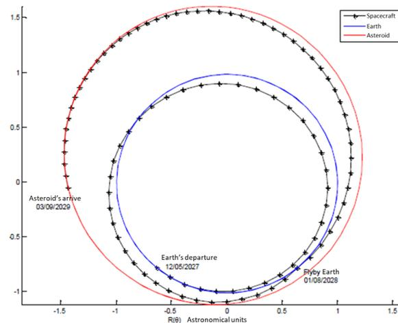
Figure 1: Example of a low-thrust interplanetary trajectory using gravity assisted maneuvers [4]
