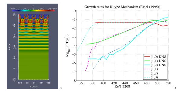
Figure 1: a. Three dimensional vortical structures generated in the K-type transition mechanism b.Growth rates of isolated modes. mechanism.
