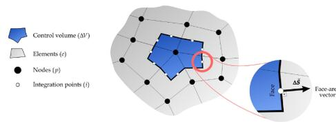
Figure 1: Main geometrical entities on the element-based finite-volume method
