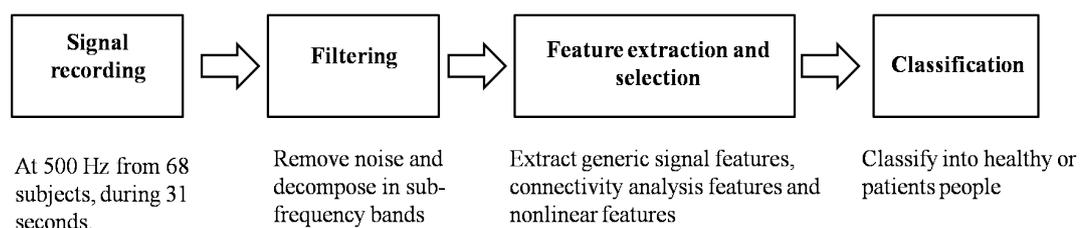
Figure 1: The classification procedure of EEG signals.
