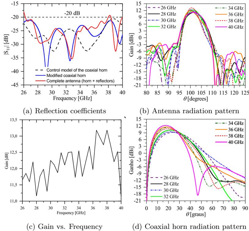
Figure 1: Antenna and feeder parameters
