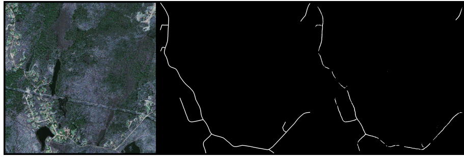
Figure 1: UNet segmentation, 20 epochs training. left: simulated SAR, center: ground truth mask, right: predicted mask. Source: authors.
